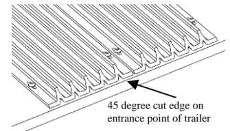
**STEP 3:** At the non-slotted end of each glide, place a screw through each outer flange 1" in from the end of each glide. The remaining screws and bushings will go into the slots. Place them in the center of each slot. This, along with the 3/8" gap between glides, allows the glides to expand and contract in various temperatures without buckling.
