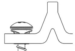
**NOTE:** Pre-drilling holes for the screws in the glides or trailer are not required if the trailer deck is wood. The screws supplied with this kit are not meant to be used in steel or aluminum, but can be if an 11/64" drill bit is used first to drill a pilot hole. Caution should be used in areas where marker lights and wires have been installed under the trailer deck when installing all fastener.
