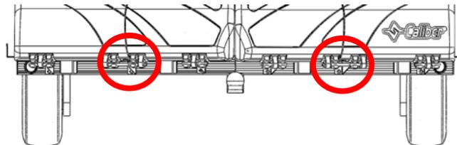
**STEP 3:** Add Rubber support strap half way up the shield. Exact Location is flexible as long as both strap and receptacle bracket on strap are lined up horizontal. Make sure receptacle bracket curve wraps around inside corner of shield panel. Drill 7/32" holes in the shield and fasten with provided rivets
