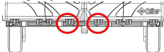
**STEP 2:** Replace middle 2 brackets in the center of each shield half with the provided Short Slotted replacement SS brackets. Use existing bolts provided with shield hardware kit. Shields existing non-slotted brackets will be used on edge of trailer. Discard remaining for non slotted brackets.
