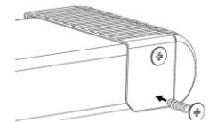
**Step 5:** Centerboard on inside of wrap upside down (if bunk board is removed from trailer or lift) Fold bunk wrap around bunk and end caps while checking length center alignment. Screw and snitch in middle 2 fastening points (or closest slot)
