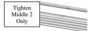
**Step 6:** Continue adding fasteners in all slots (every 12”) but leave a small 1/16” gap between fastening head and material “DO NOT TIGHTEN” this will allow material to expand and contract with different temperatures eliminating any ripples or bowing in your bunk wrap.
