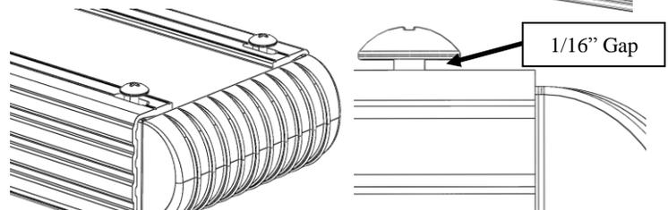
**Step 7:** Reattach bunk boards on Trailer Bracket mounts. Trim away any interfering material so bracket sits directly on wood. If existing holes are stripped move slightly and relocate for secure fastening.
