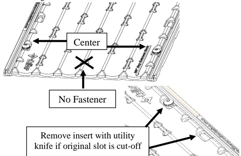
**NOTE:** The screws supplied with this kit are not meant to be used in steel or aluminum, but can be if an 11/64" drill bit is used first to drill a pilot hole. Caution should be used in areas where marker lights and wires have been installed under the trailer deck when installing all fastener.
