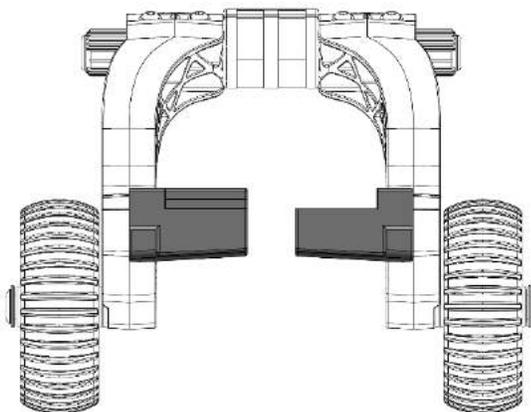
3b. For skis with uneven keels or carbides (i.e. SkiDoo Pilot skis and others), use a finger extender (17 and 18) as before, but cut the extender on the carbide side of the ski using a sharp blade. Use the horizontal lines on the extenders as a guide. Tap the rubber on a hard surface to ensure it is fully seated. Secure with self-tapping screws (19). This will make your Sled Wheels left or right handed, so be sure to use them on the correct ski, or your skis will not sit flat.
