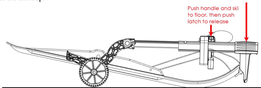
2. Slowly move the handle up. Remove Sled Wheels from the ski, lifting the ski loop if necessary. Close latch and replace safety pin. Store fully assembled, ready for your next ride!
