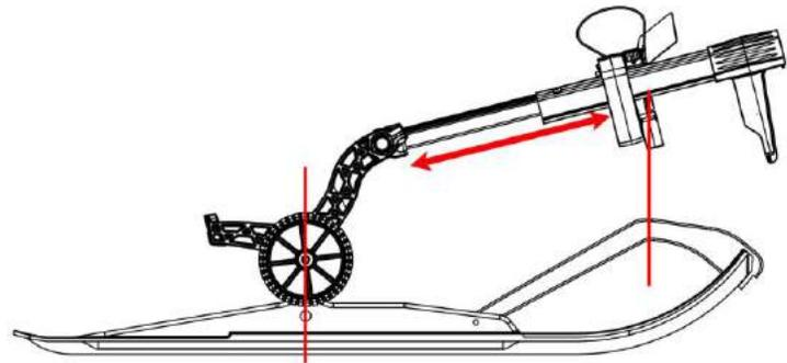
5. Loosen the latch adjustment screw three turns so that the lower portion of the latch is moveable. Slide the latch all the way down.
