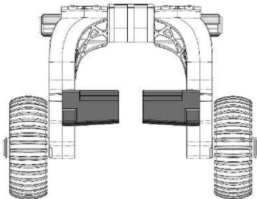
3a. For skis that are flat or have even guides, assemble the finger extenders (17 and 18 - be sure to use the left cover on the left arm, and right on right). Tap the rubber on a hard surface to ensure it is fully seated. Secure with a self-tapping screw (19).
