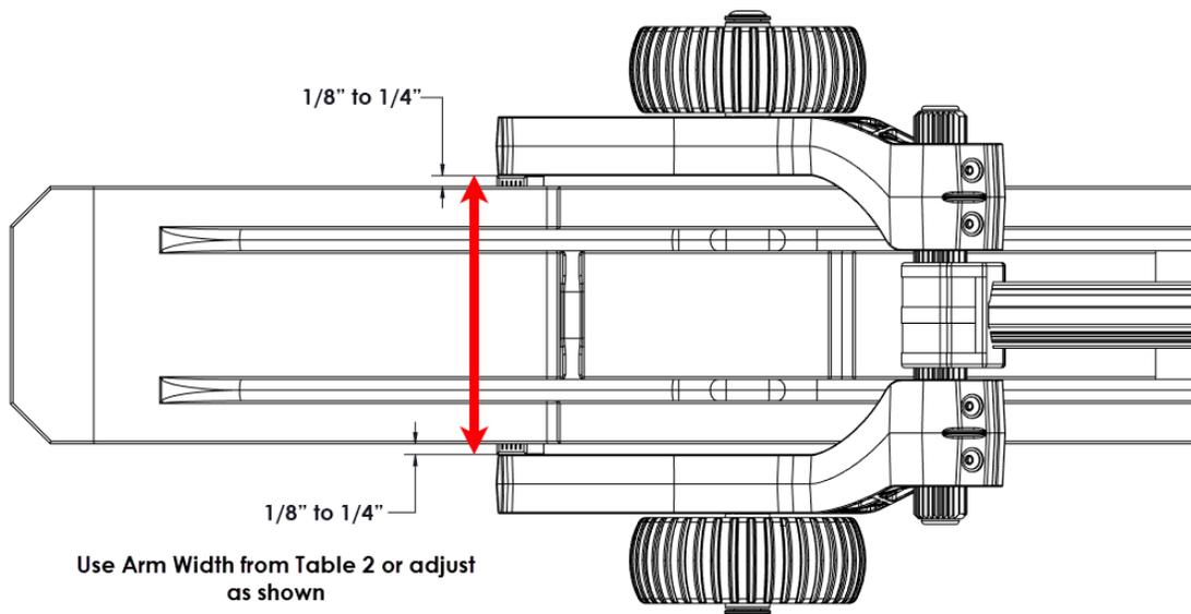
3. Position one Sled Wheel assembly above the ski so that the Sled Wheels axle is directly above the ski spindle axle. Loosen the Telescoping handle screw and move the handle so it hits the end of the ski. Tighten the screw (approximately 4 ft-lbs).
