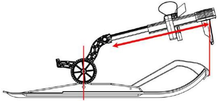
4. Adjust the saddle/latch assembly so that the latch will close at the peak of the ski loop. Tighten the saddle screw (approximately 4 ft-lbs).
